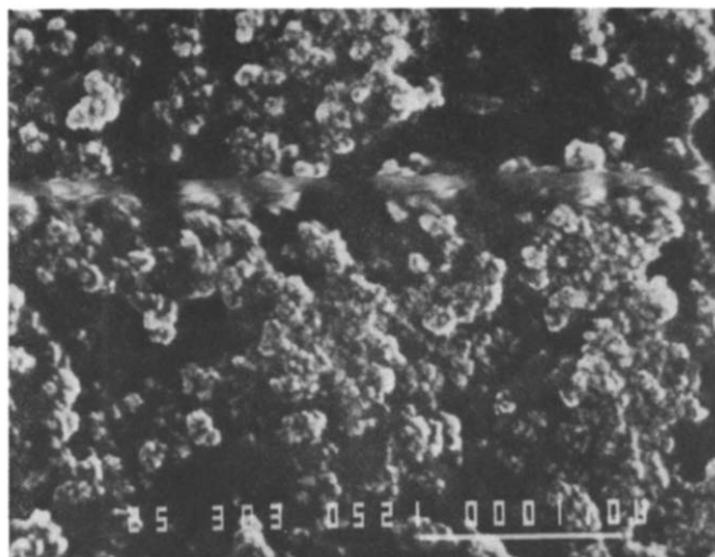
Figure 5 Cross-section of film shown in Figure 2 coated with \sim 80 \text{ \AA} evaporated gold
